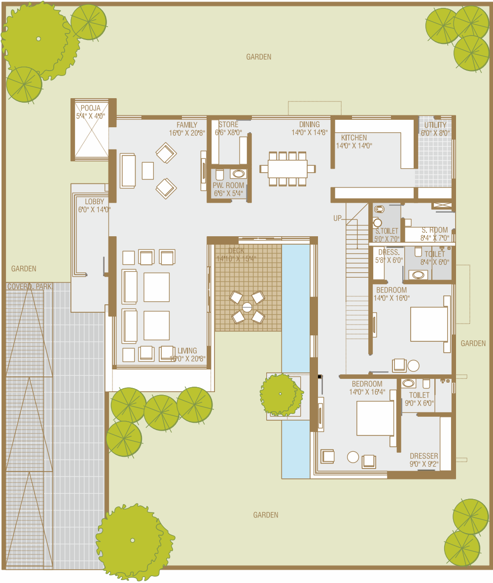
TYPE E GROUND FLOOR PLAN BUILT UP AREA = 269.82 SQ.M (2904 SQ.FT.)
